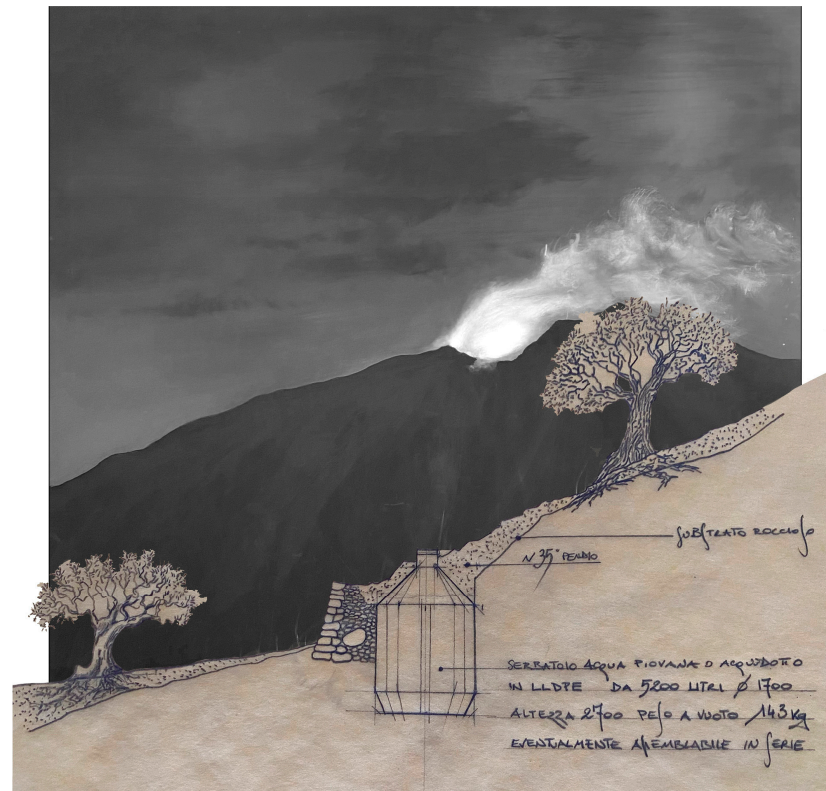
Figure 5. Section of the water harvesting device integrated into terraces dedicated to olive cultivation. The handwritten text in the drawing outlines the main technical characteristics of a rainwater tank installed on a 35° slope over a rocky substrate. The tank is constructed from LLPDE (linear low-density polyethylene) and has a capacity of 5200 liters (diameter 170 cm, height 270 cm; empty weight 143 kg). It can possibly be assembled in series. The design also features the volcano in the background (credit, F.V.C.).
