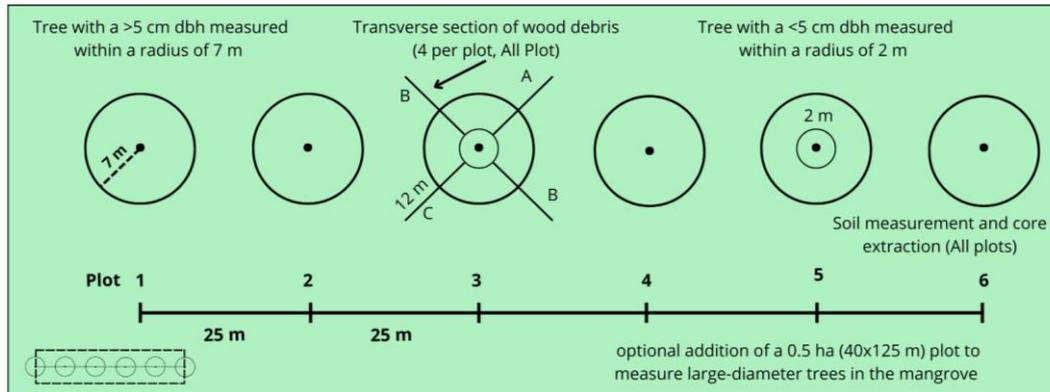
**Figure 2.** Standard plot design and size for measuring mangrove forest carbon stocks [13].
