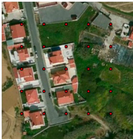
Figure 2. An example of a PSU (area of the image) and SSUs (red dots) within. SSUs are organized in a 20 m grid (25 sampling points) to assess impervious surfaces implemented by the CLMS service providers in the validation of the IMD layers.
