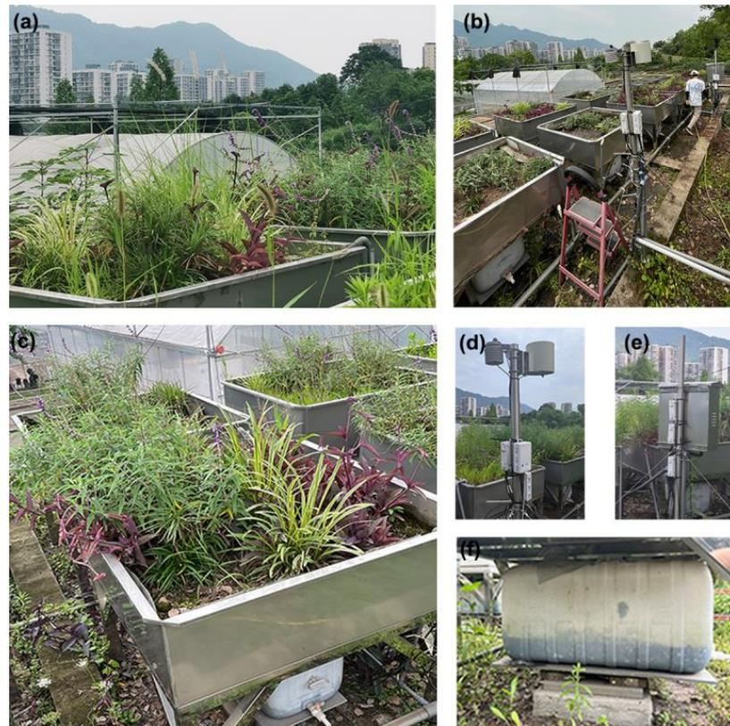
Figure 2. (a) Green roof modules situated on an open platform. (b) An overview of the module arrays immediately following the initial planting phase. (c) A single green roof module. (d) Meteorological instruments positioned alongside the green roof modules. (e) Data logger positioned next to the green roof modules. (f) A runoff collection container beneath a module.
