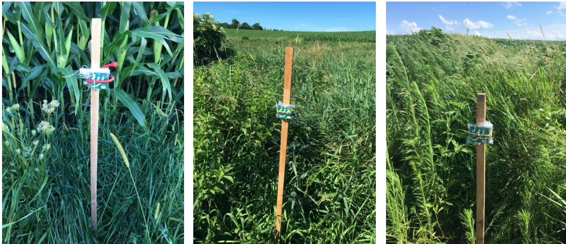
Figure S1. Photographs of AudioMoth passive acoustic monitors deployed in the field.
