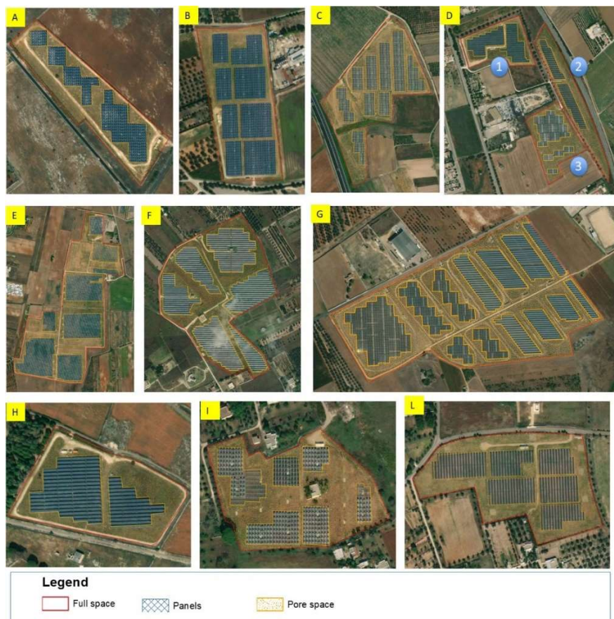
Figure 4. Characterisation of pore spaces in some GPV systems (A–L) located in the Apulia region (southern Italy), in the provinces of Brindisi and Lecce. Please see Table 2 for the description of the systems.
