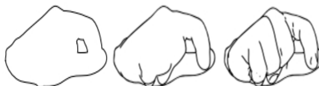
Figure 2. A sample of the rendered silhouette ( left ), occluding contours ( center ), and suggestive contours ( right ).
