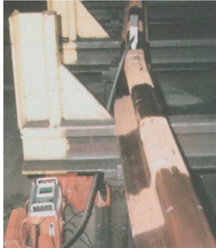
Figure 14. Measurement of residual stress with a DEBRO instrument.
