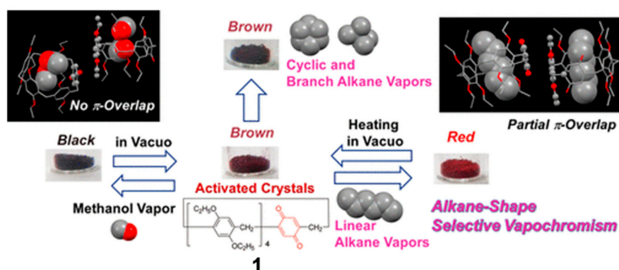
Figure 1. Vapochromic behavior of 1 against various alkane vapors and methanol vapors. Reproduced with permission from Reference [20]. Copyright 2017 American Chemical Society.
