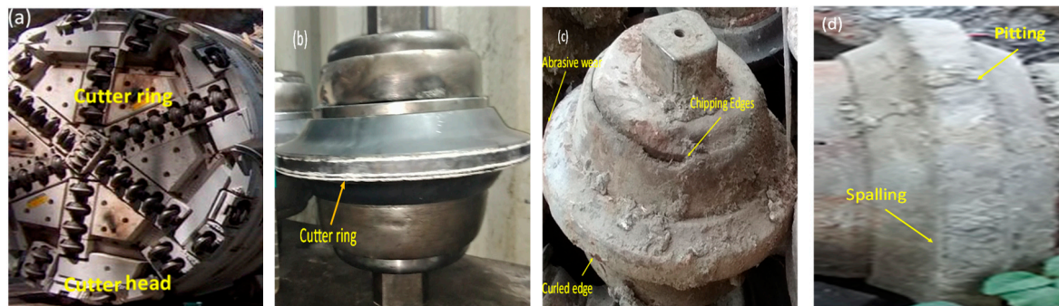
Figure 1. (a) cutter head with cutter rings; (b) new cutter ring; (c,d) worn out cutter rings.
