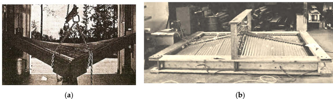
Figure 8. Two symmetric experimental hyperbolic paraboloid shells: (a) a single shell by McDermott [17]; (b) an umbrella structure of four quarters by Banavalkar and Parker [16].
