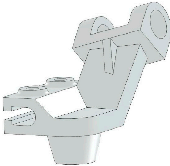
Figure 5. This is an example of a part with a nerve whose placement would be much easier if based on the bisecting plane concept.
