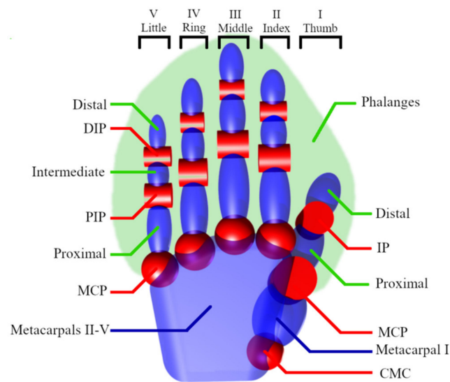
Figure 1. Proximal Interphalangeal (PIP), Distal Interphalangeal (DIP) and Metacarpophalangeal (MCP) connected to Metacarpals I joint have one axis of rotation, while the MCPs connected to Metacarpals II-V and Carpo-Metacarpal (CMC) joints have two axes of rotation.
