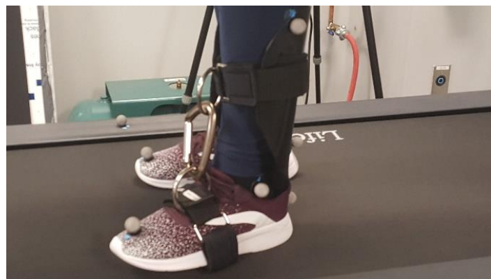
Figure 1. Brace designed to restrict ankle range of motion by opposing plantarflexion.
