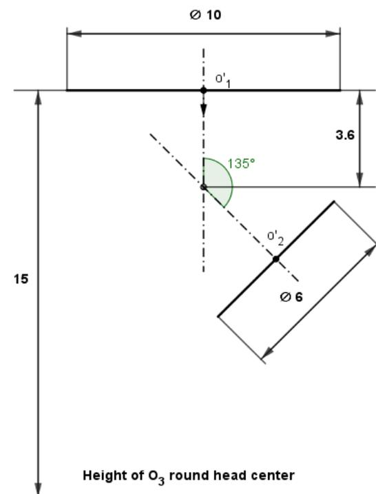
**Figure 2.** Orthographic projection with reference dimensions (m) of round mouths (centers  $O_1$ ,  $O_2$ ) of tronco-conic hopper and relative height of the connected round head center ( $O_3$ , see text).
