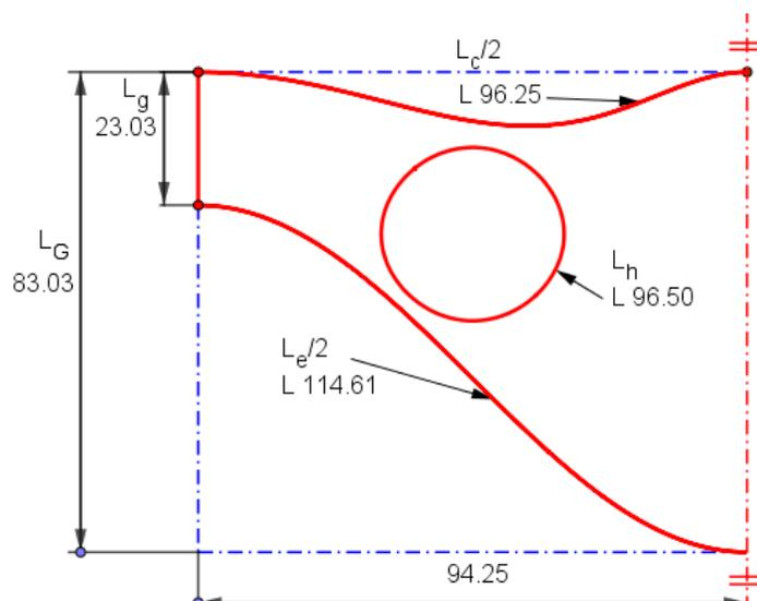
**Figure 5.** Dimensioned (cm) half-pattern of the 4-way cylindrical hopper obtained by CEDG approach for the reference parameters' values.
