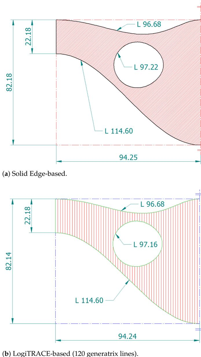
**Figure 4.** Half-patterns of the 4-way cylindrical hopper obtained by computer-aided design (CAD) approaches for the reference parameters' values. Dimensions are in cm.
