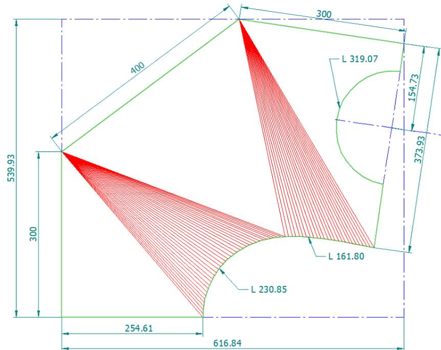
**Figure 10.** Dimensioned (mm) half-pattern of the Round-poligonal transformer with circular branch obtained by LogiTRACE approach with 120 generatrix lines for the reference parameters' values.
