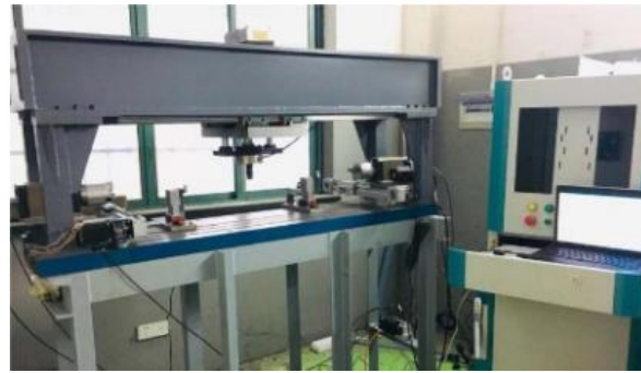
Figure 6. Main worktable of hexagonal shaft straightening machine.
