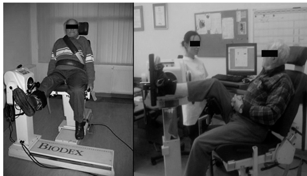
Figure 4. Measurement of force-velocity parameters of flexor and extensor muscles of the knee and ankle (Biodex System 4; own source).
