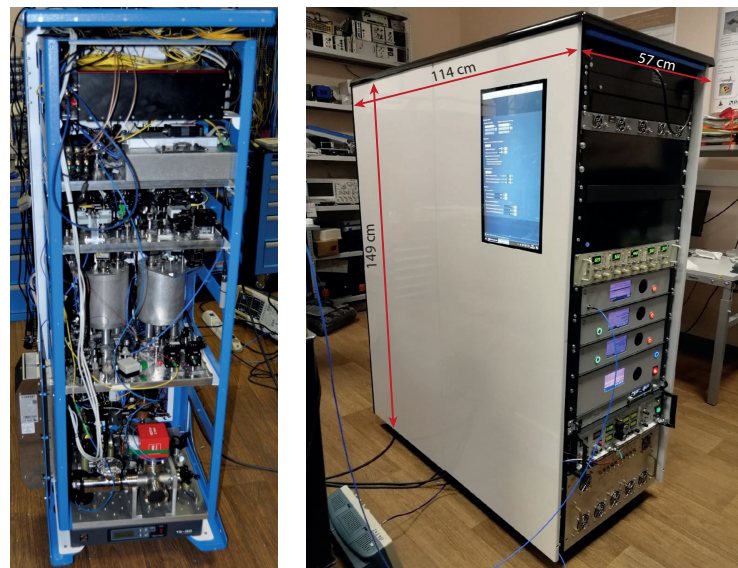
Figure 1. The first generation of a transportable single ^{171}\text{Yb}^+ clock at the Lebedev Institute.
