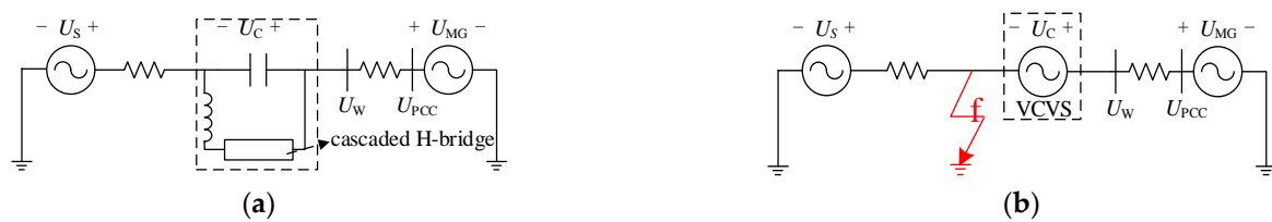
Figure 2. Schematic diagram of the CHB-FFCL voltage regulation principle (single-phase). (a) Grid connection diagram of the CHB-FFCL. (b) Equivalent circuit diagram of when a fault occurs.
