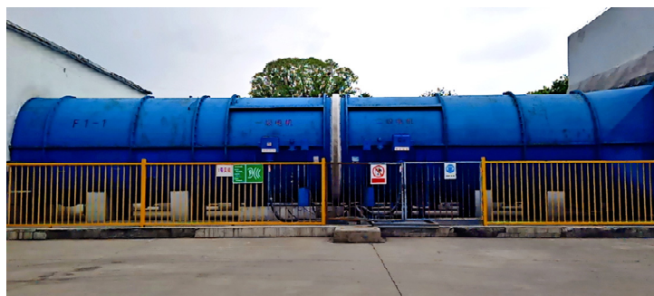
Figure 7. FBCDZ-8-No34 counter-rotating axial flow coal mine main fan.
