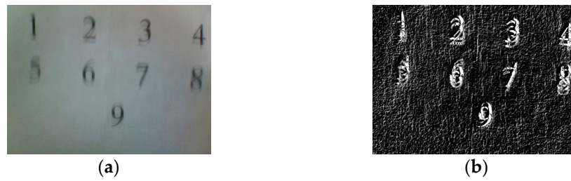
Figure 14. (a) Input image; (b) Sobel operator at 260 lux.
