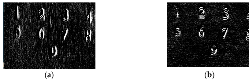
Figure 15. (a) Sobel operator on the x -axis; (b) Sobel operator on the y -axis at 260 lux.
