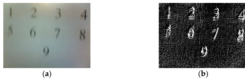
Figure 10. (a) Input image; (b) Sobel operator at 100 lux.
