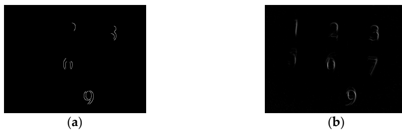
Figure 4. (a) Canny's operator; (b) Prewitt's operator at 70 lux.
