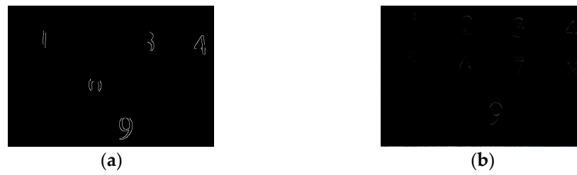
Figure 8. (a) Canny operator; (b) Prewitt's operator on the y -axis at 50 lux.
