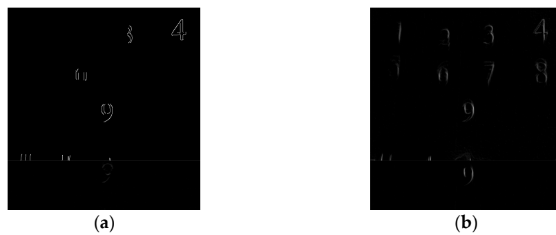
Figure 28. (a) Canny operator; (b) Prewitt's operator at 2350 lux.
