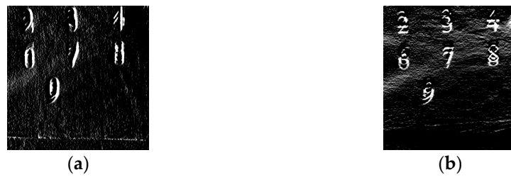
Figure 19. (a) Sobel operator on the x -axis; (b) Sobel operator on the y -axis at 2300 lux.
