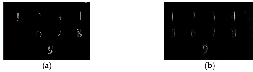
Figure 24. (a) Canny operator; (b) Prewitt's operator at 2300 lux+ man shadow.
