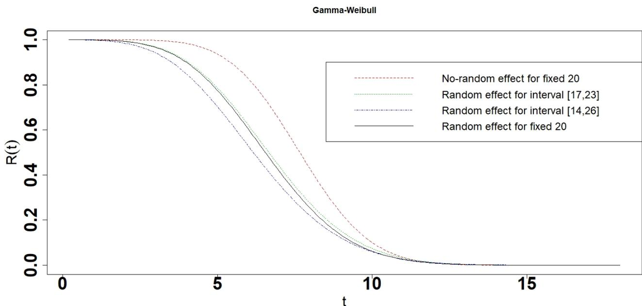
**Figure 31.** Reliability of the photovoltaic module for the Gamma-Weibull interval degradation model.
