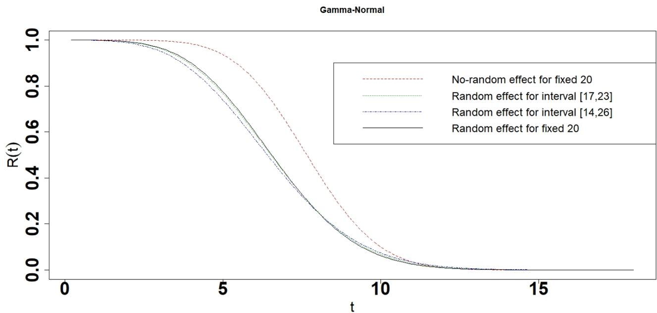
Figure 28. Reliability of the photovoltaic module for the Gamma-Normal interval degradation model.
