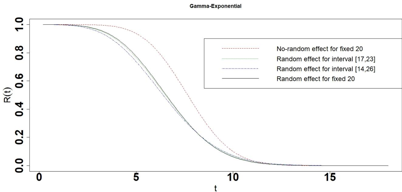
**Figure 30.** Reliability of the photovoltaic module for the Gamma-Exponential interval degradation model.
