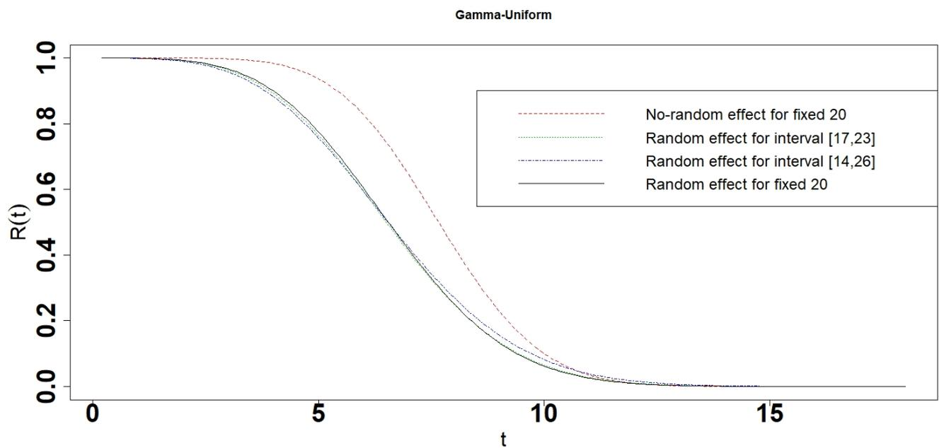
Figure 29. Reliability of the photovoltaic module for the Gamma-Uniform interval degradation model.
