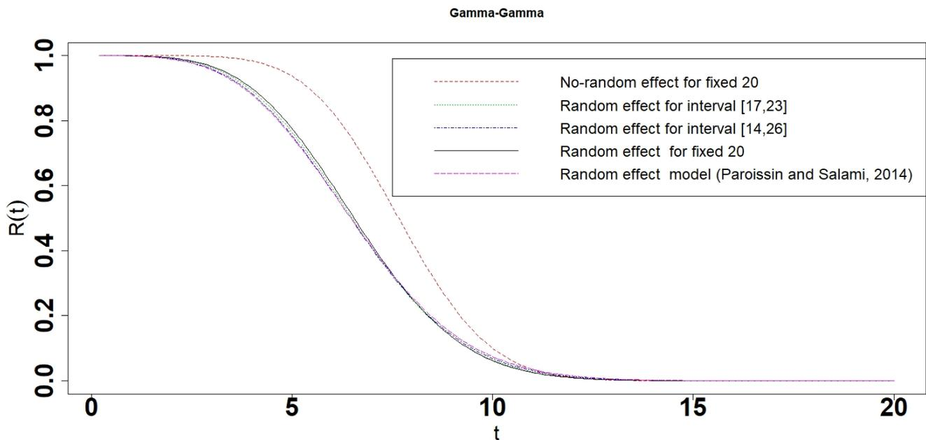
**Figure 27.** Reliability of the photovoltaic module for the Gamma-Gamma interval degradation model.
