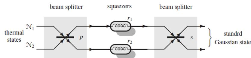
**Figure 1.** Implementation of a two-mode Gaussian state with the covariance matrix in *standard form*.
