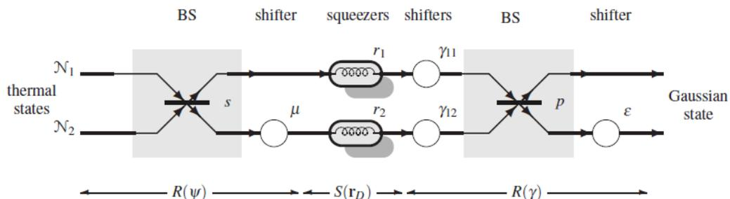
**Figure 4.** Scheme with primitive components for the generation of a general two-mode Gaussian state, starting from two thermal states,  $\mathcal{N}_1$  and  $\mathcal{N}_2$ . The architecture does not contain the irrelevant initial rotations  $\psi_{11}$  and  $\psi_{12}$  and the final displacements  $\alpha_1$  and  $\alpha_2$ , which do not influence the covariance matrix.
