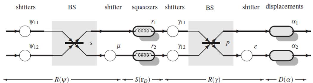
**Figure 3.** Implementation of a general two-mode Gaussian unitary with primitive components.
