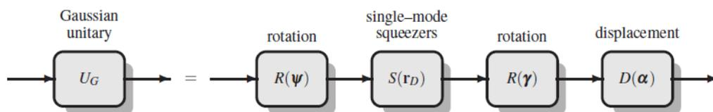
Figure 2. Decomposition of a Gaussian unitary according to the Bloch–Messiah (BM) reduction.
