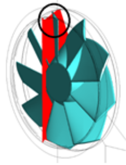
Figure 13. Impeller eccentricity diagram.
