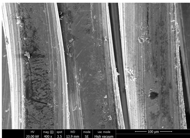
(c) MR-3 after creep test at 250 °C
