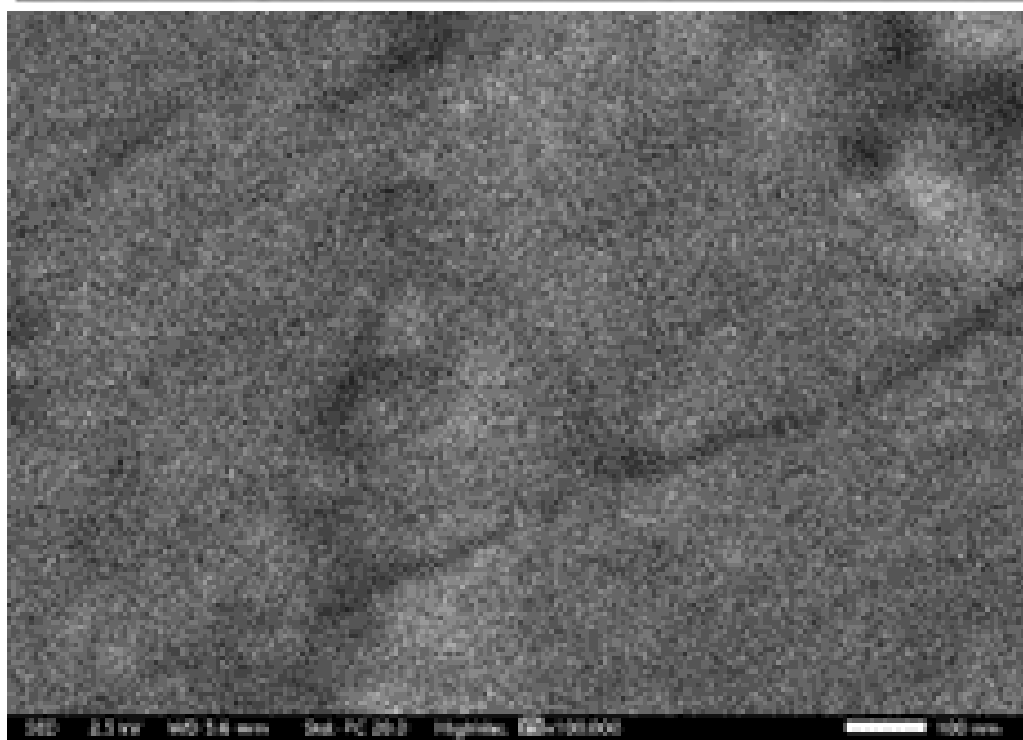
Figure S7. SEM images of the polymer surfaces obtained by CPE at 0.6 V, 4 mC (14 mC/cm 2 ) (CME 14) at two magnifications: x300, 5 kV (a) and x10 5 , 2.5 kV (b).
