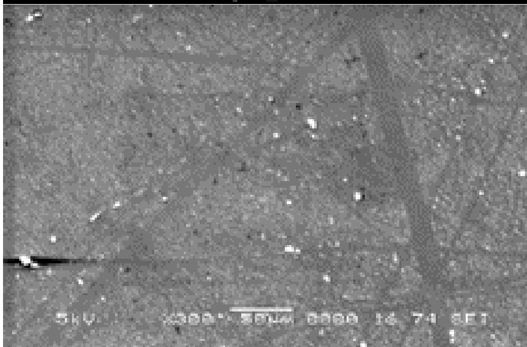
Figure S8. SEM images of the polymer surfaces obtained by CPE at 0.6 V, 8 mC (28 mC/cm 2 ) (CME 15) at two magnifications: x300, 5 kV (a) and x10 5 , 2.5 kV (b).
