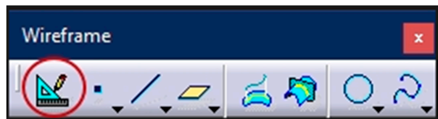
Figure 1. Shortcut icon (red circle) from the “Wireframe and Surface Design” module toolbar.
