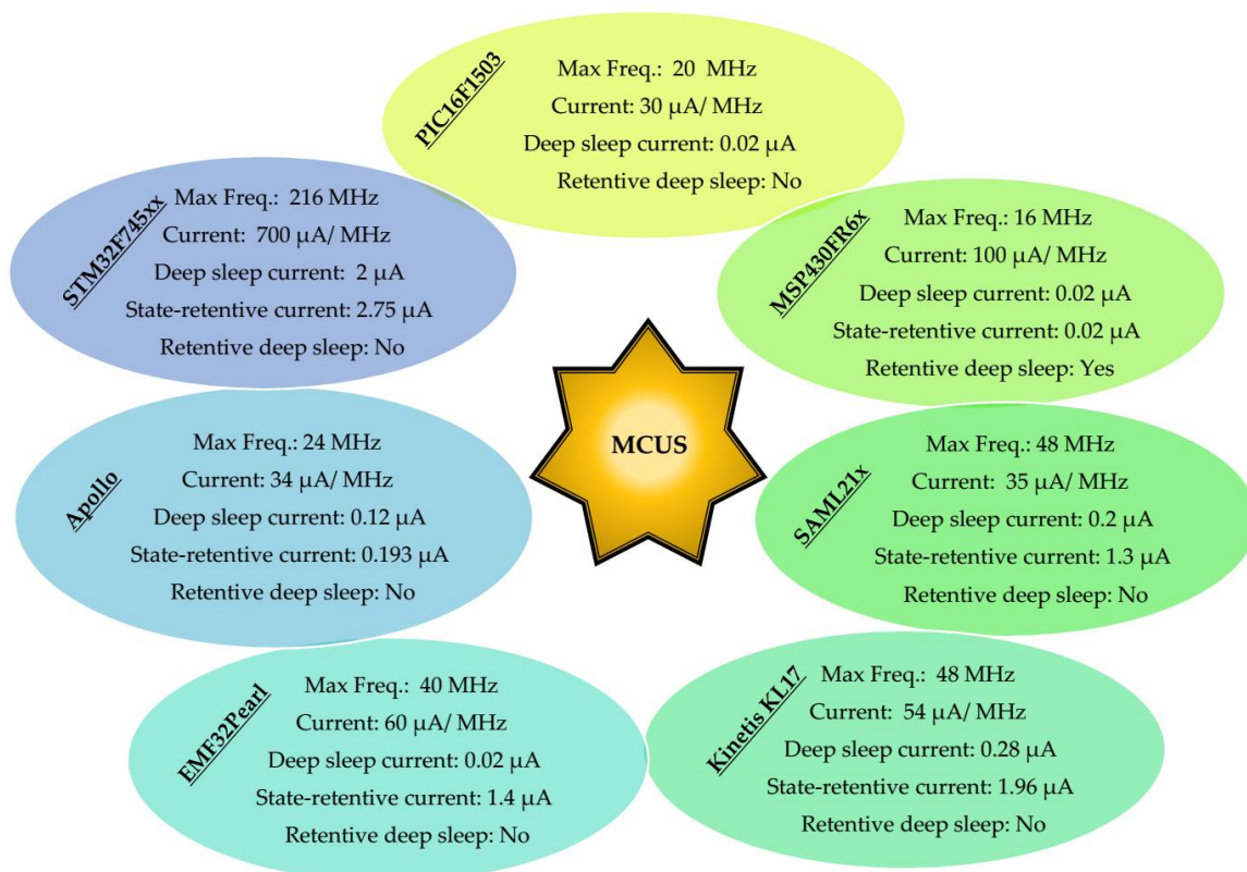
Figure 16. A summary of the key characteristics of MCUs commonly employed in ultra-low power applications.
