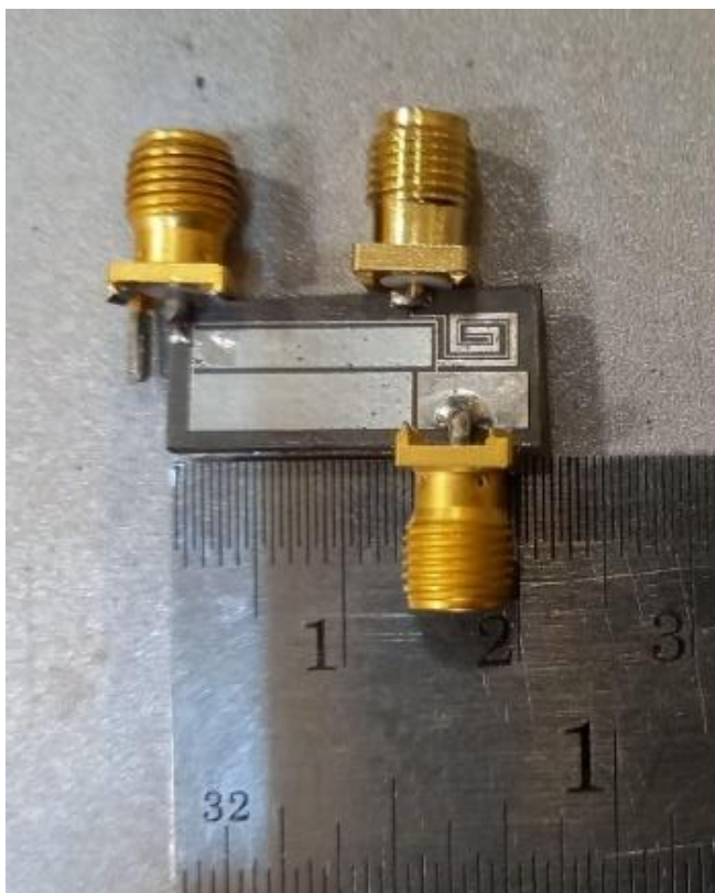
Figure 6. Three-channel diplexer with the dimensions in mm with a photograph of the fabricated diplexer.
