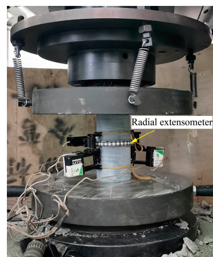
(b) MTS STH GB-T universal testing machine
