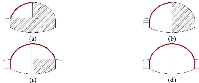
Figure 6. Schematic diagram of bench excavation and support.
