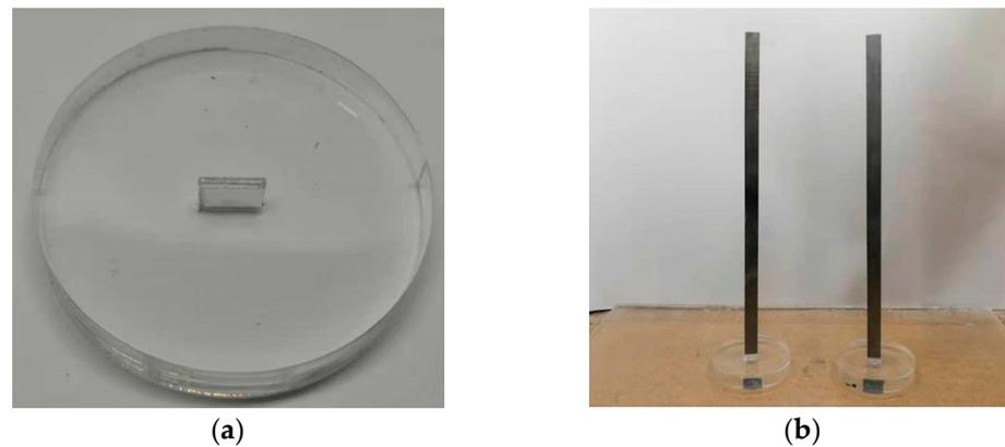
**Figure 4.** Prefabricated crack mould, (a) resin base, (b) steel sheet.
