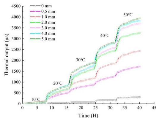
**Figure 9.** Relationship of temperature to thermal output for different paste thicknesses of the adhesive layer.
