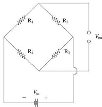
Figure 1. Wheatstone bridge circuit.
