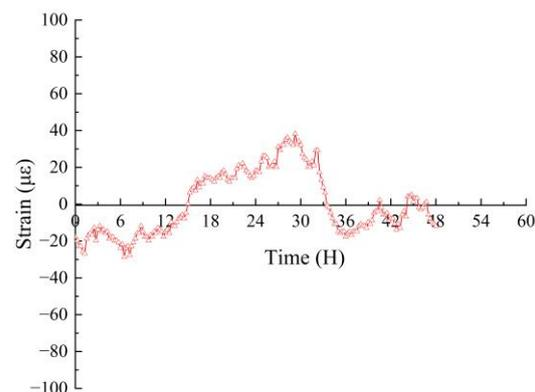
**Figure 2.** The “zero drift” data for a strain gauge.
