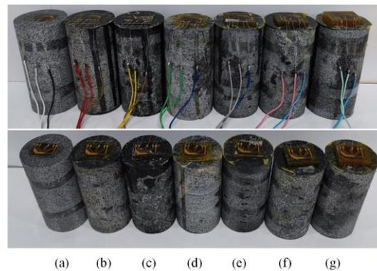
**Figure 8.** Strain gauges pasted on adhesive layers with different thicknesses: (a) 0; (b) 0.5 mm; (c) 1.0 mm; (d) 2.0 mm; (e) 3.0 mm; (f) 4.0 mm; (g) 5.0 mm.
