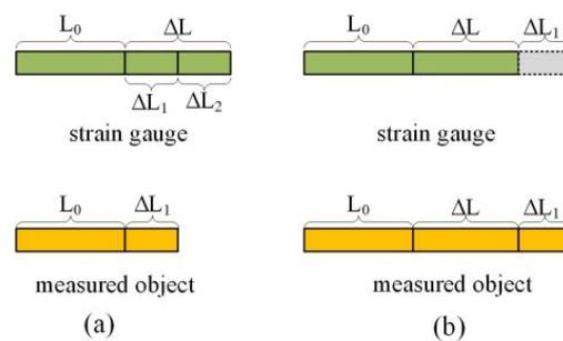
**Figure 7.** Coupled deformation of strain gauges and measured materials during temperature change: (a)  $\alpha_s < \alpha_g$ ; (b)  $\alpha_s > \alpha_g$ .
