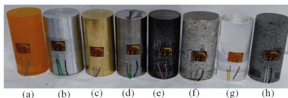
**Figure 3.** Strain gauges pasted on measured materials with different linear expansion coefficients: (a) epoxy resin adhesive, (b) aluminum, (c) brass, (d) stainless steel, (e) iron, (f) concrete, (g) plexiglass, and (h) granite.
