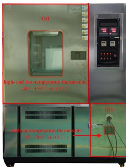
**Figure 4.** Thermostats with dual temperatures. (a) high- and low-temperature thermostats:  $-40\sim 150^\circ\text{C}$  ( $\pm 0.1^\circ\text{C}$ ); (b) Ambient temperature thermostats:  $15\sim 50^\circ\text{C}$  ( $\pm 0.1^\circ\text{C}$ ).
