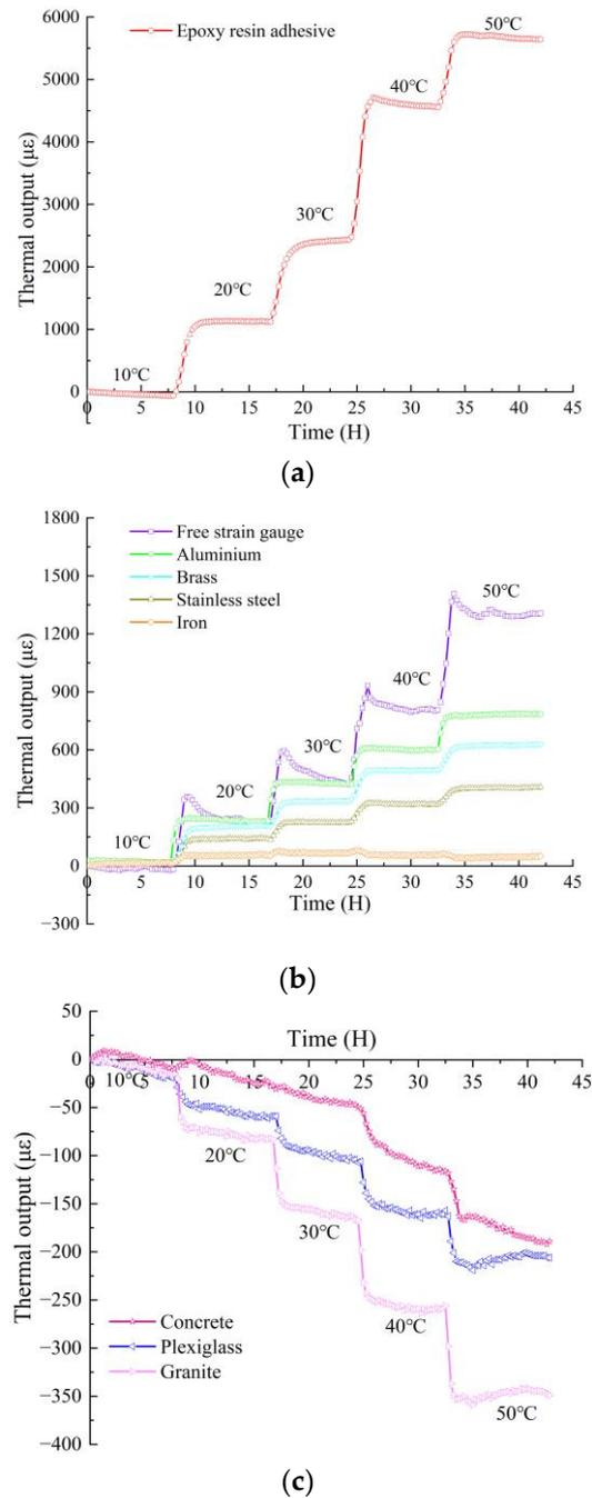
**Figure 5.** Thermal output of the strain gauges pasted onto different materials: (a) epoxy resin adhesive; (b) free strain gauge, aluminum, brass, stainless steel, iron; (c) concrete, plexiglass, granite.
