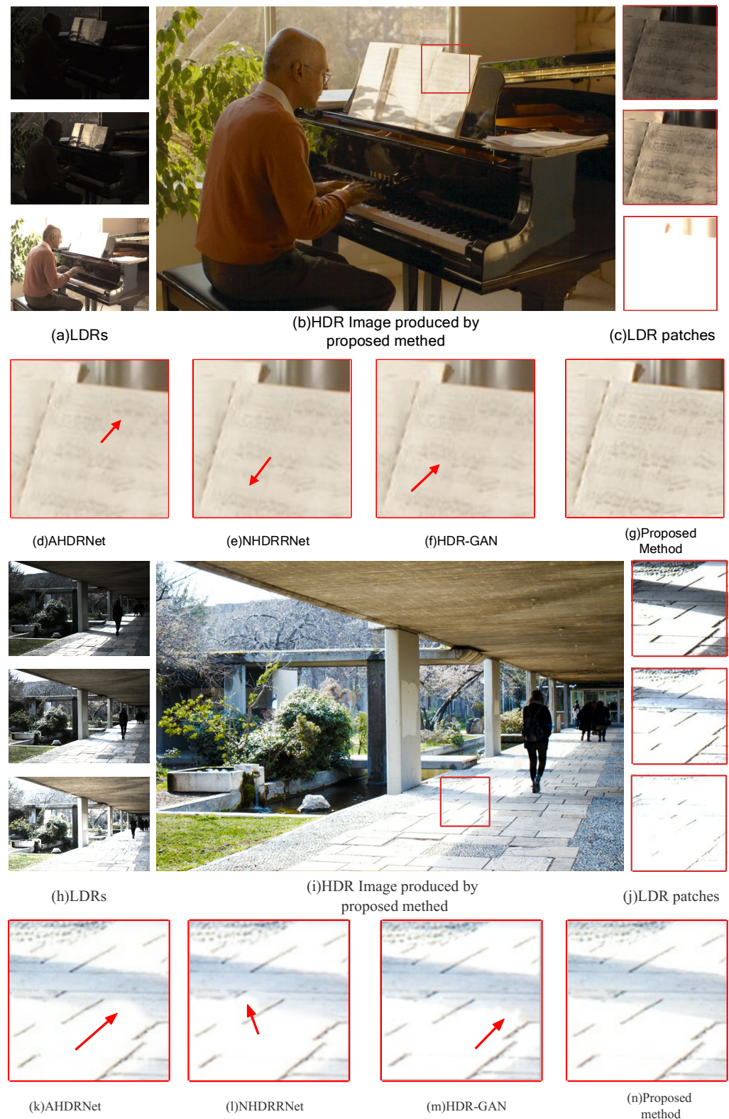
Figure 8. The comparison results from the sen/tursun dataset (which does not provide GT images) were subjectively compared with images generated by other SOTA methods [6,8,12] after TM, and partial comparison area results were presented. The red arrows indicate the compositional differences in the comparison methods.
