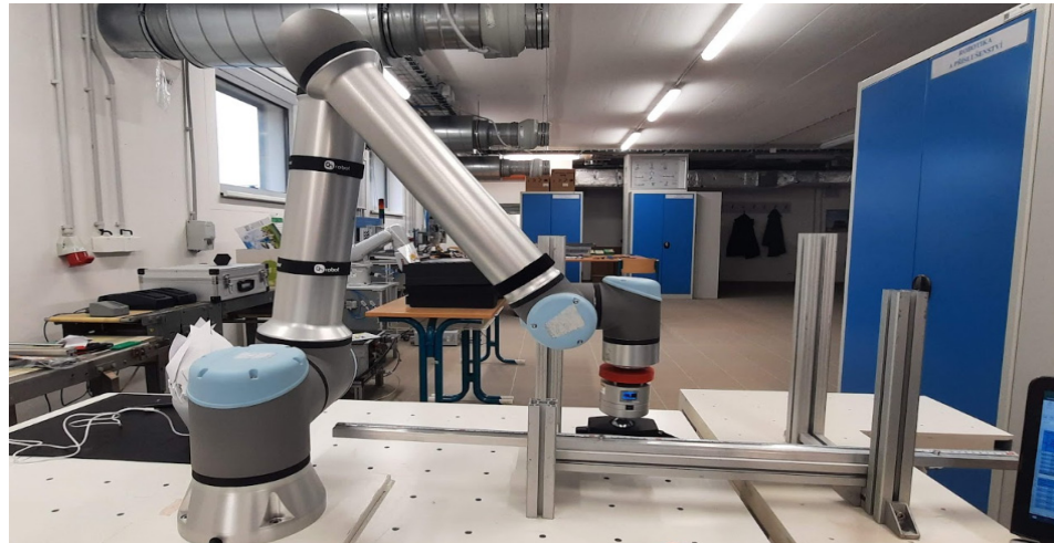
Figure 7. Position of UR arm joints in collision in coordinate [450; 200].
