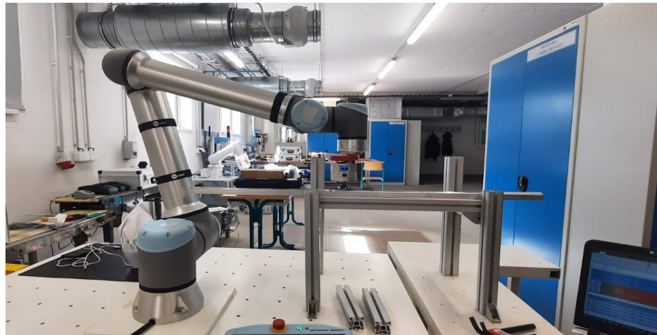
Figure 11. Position of the UR10 arm joints in a collision in coordinate [450; 500].
