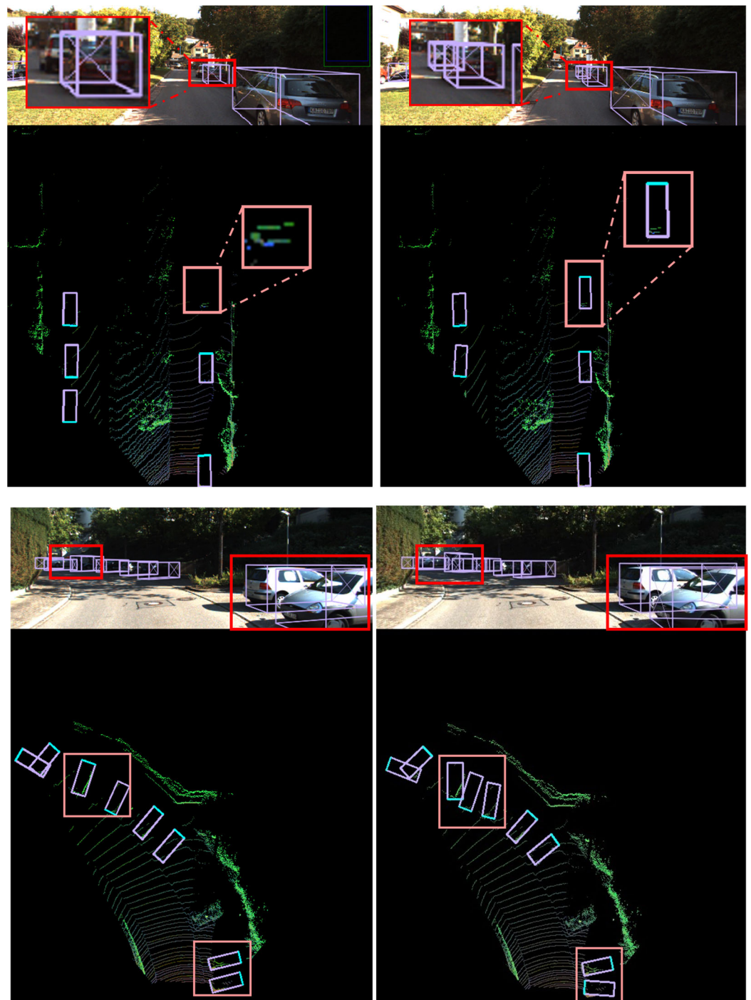
Figure 9. Visualization comparison for partially occluded-object-detection results with PointPillars ( left ) and our 2SFNet ( right ). Notice that predictions are entirely based on BEV maps derived from point clouds. Re-projecting to image space is for illustrative purposes only.
