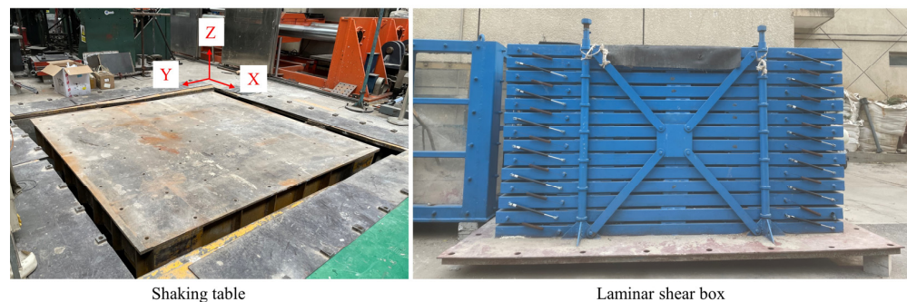
Figure 2. Shaking table and model box.
