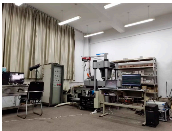
Figure 6. Rock shear seepage meter.
