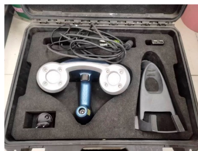
Figure 22. Handheld 3D laser scanner.
