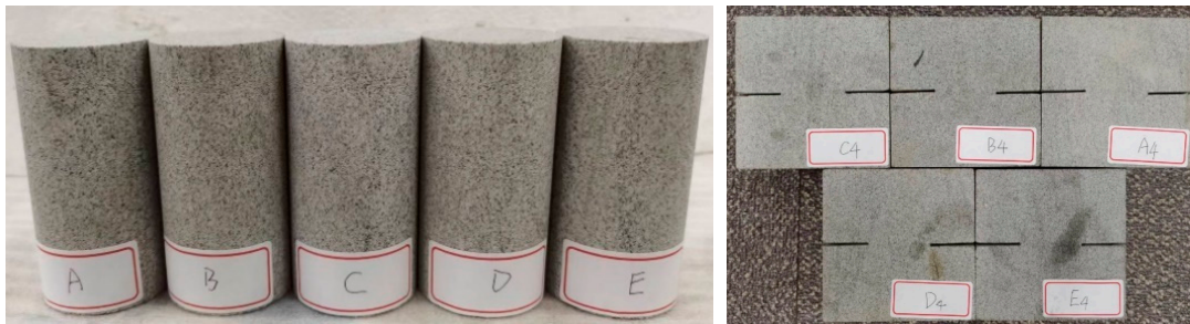
Figure 7. Rock mass specimens after different numbers of freeze–thaw cycles.
