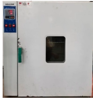
Figure 2. Electric blast drying oven.
