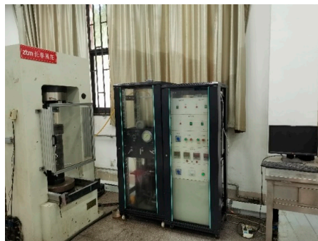
Figure 4. Triaxial testing machine.
