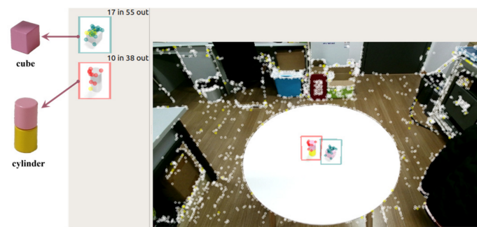
Figure 18. Kinect2 recognizes the items to be picked up.
