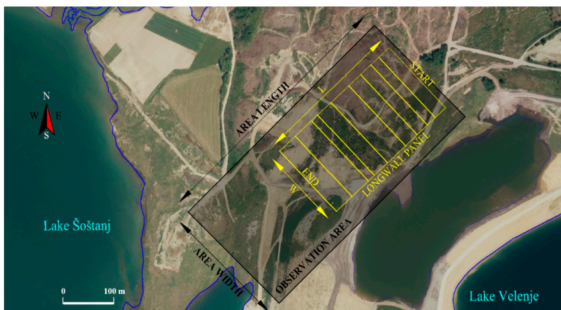
Figure 3. The discussed longwall panel excavation in the observation area.
