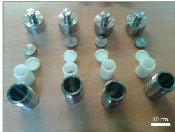
**Figure 2.** Teflon vessel and reactor for hydrothermal synthesis used in the laboratory experiment.
