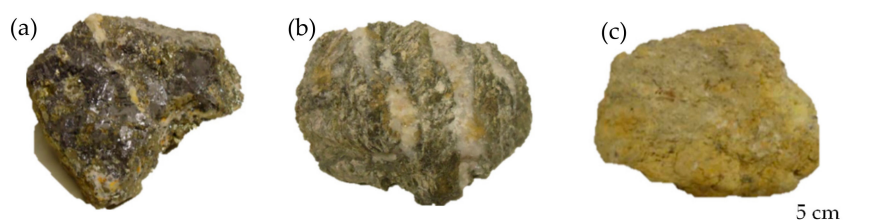
Figure 1. Photographs of some of the analysed rock chip samples, (a) ore that consists of the sulphide minerals (e.g., galena, pyrite and sphalerite); (b) host rock—banded gneiss; and (c) the weathered material (e.g., clay minerals).
