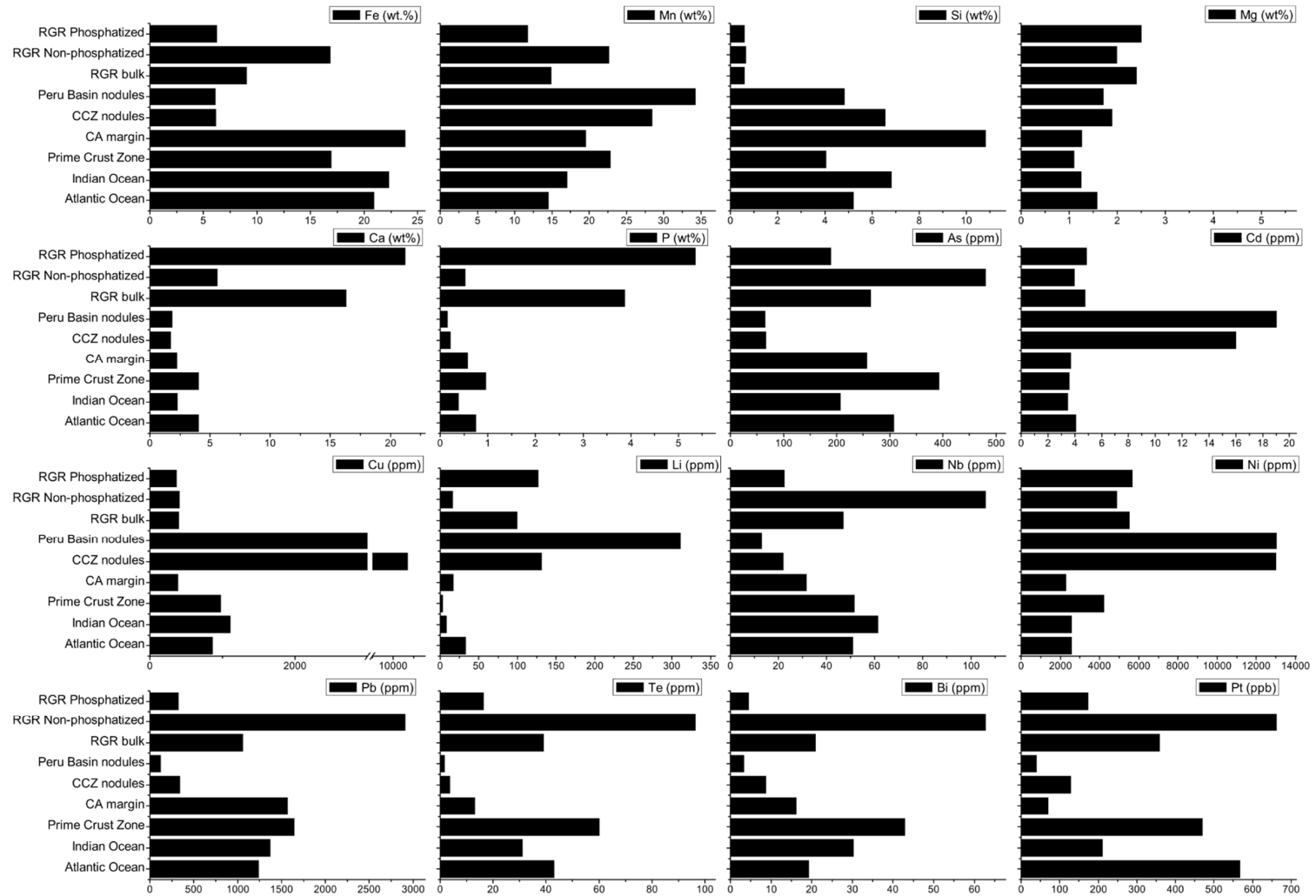
Figure 7. Comparison between the chemical composition of bulk, non-phosphatized Fe–Mn crusts, and phosphatized crusts from the RGR summit and Fe–Mn deposits formed elsewhere, compiled by [10] from [1]. Peru Basin nodules correspond to the diagenetic end-member.
