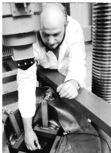
Figure 6. Sample insertion at the triaxial press.
