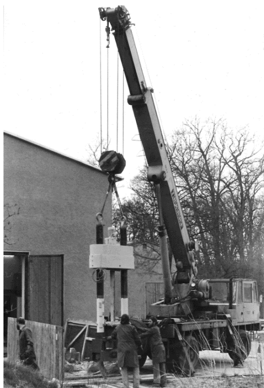
Figure 3. Assembling the triaxial press.
