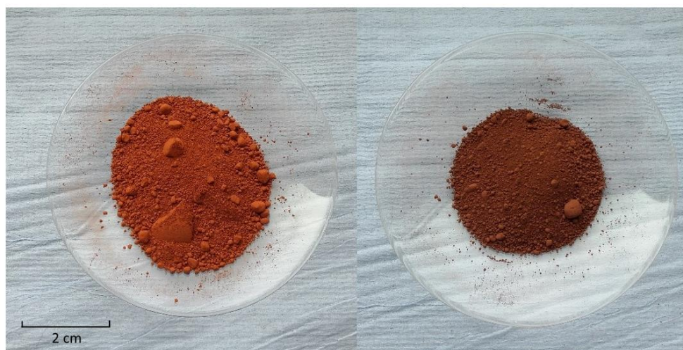
Figure 2. Red mud samples, (left) from Germany, (right) from Greece.
