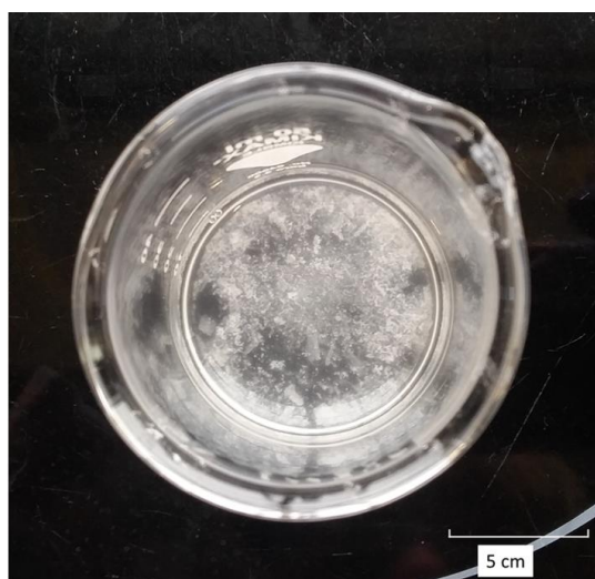
Figure 4. Typical flakes in the 5 min and 10 min samples after treatment with red mud.
