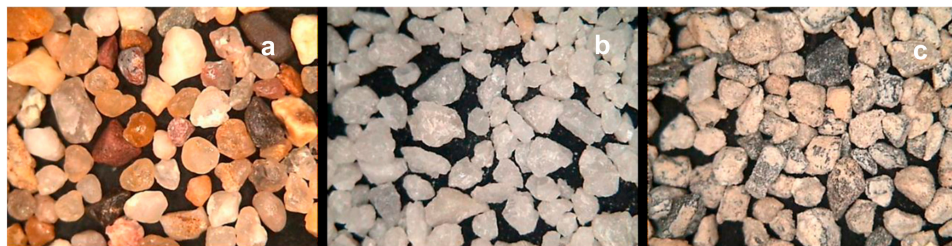
Figure 1. Image of aggregates (a) siliceous (S), (b) limestone (L), and (c) recycled aggregates (R) in fractions of maximum size 1 mm.
