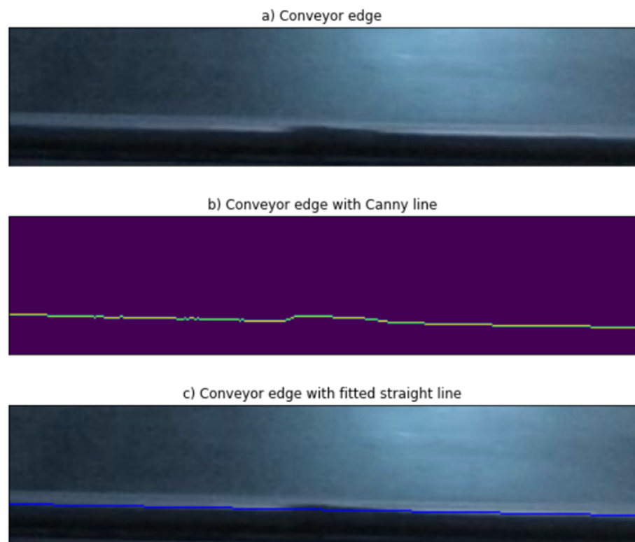
Figure 5. (a) Lower part of the conveyor belt. (b) Edge line designated by Canny algorithm. (c) Fitted straight line designated by linear regression.
