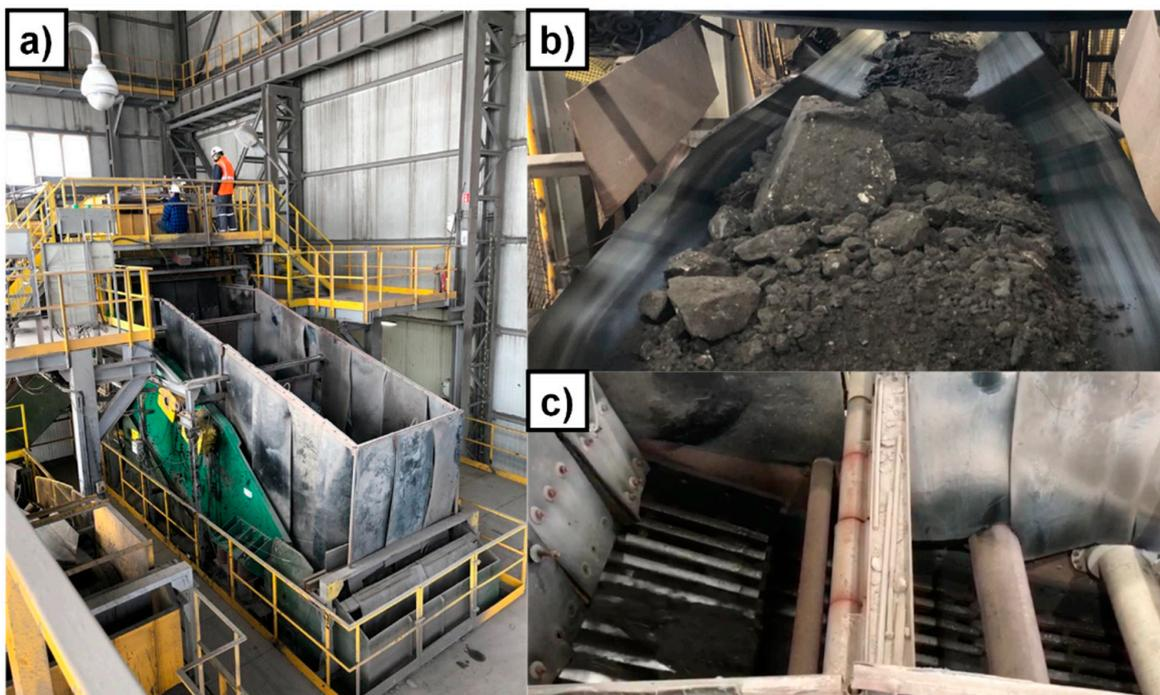
**Figure 2.** The investigated technical object—vibrating screen: (a) view of the whole device; (b) feed; (c) upper sieving deck.
