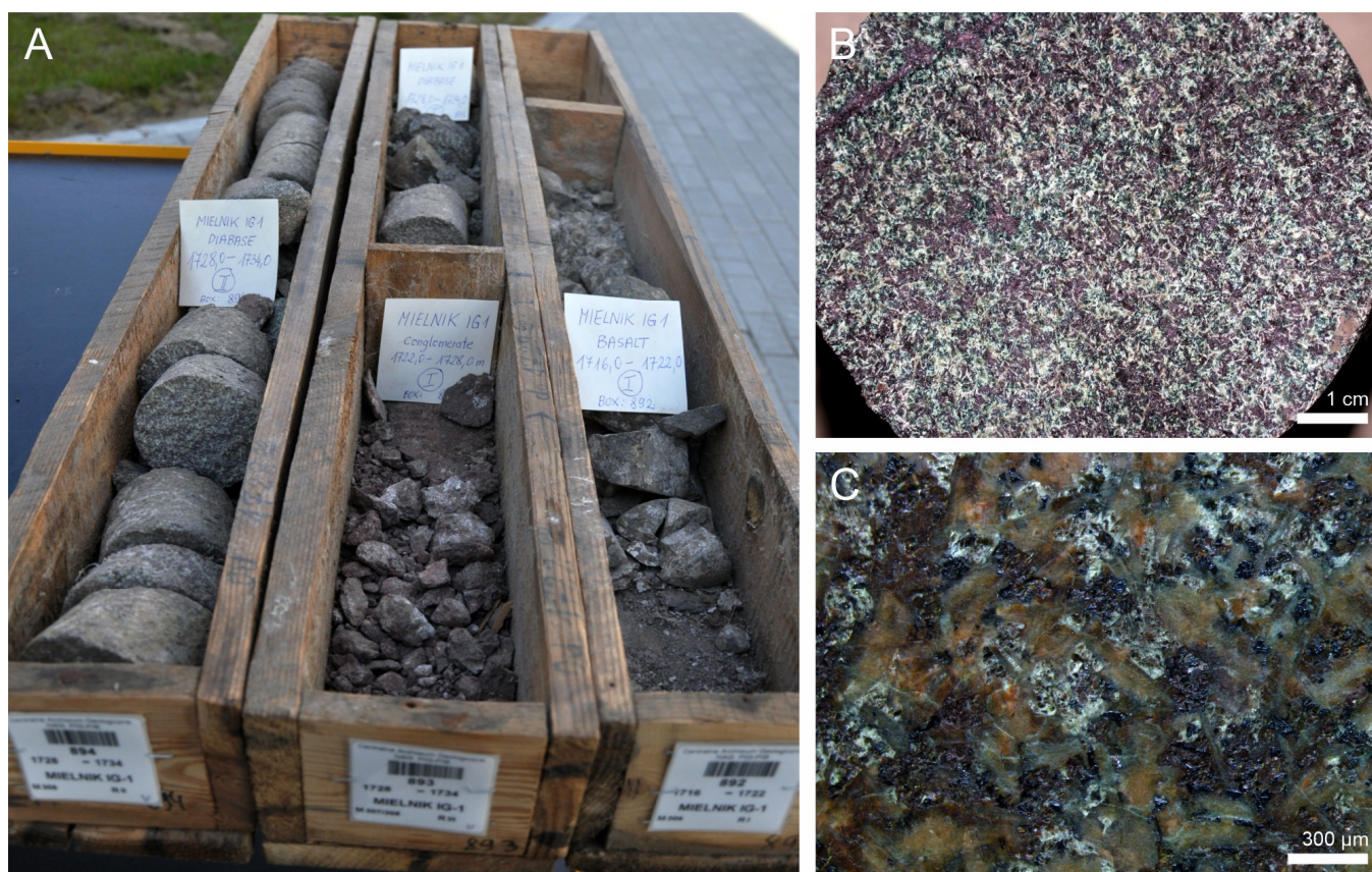
Figure 4. Photographs of the Mielnik IG1 drill cores from interval of ~1729–1722 m, showing: (A) Dolerite top (left), reduced interval of conglomerate of Żuków Formation (center) and basalts of Sławatycze Formation (right). The contacts were not retained; (B) Part of dolerite core sampled for U–Pb geochronology. Width of core is approximately 8.4 cm; (C) Dolerite rock chip (polished) to expose a poikilitic texture and main components coarse grains of plagioclase (albitized) and pyroxene and Fe–Ti oxides.
