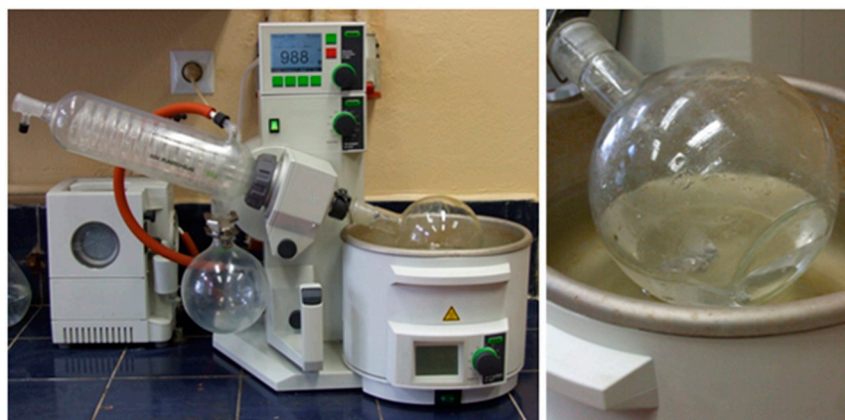
Figure 3. The rotary reactor driven by an evaporator (Buchii, Rotavapor R-210/215) used in the leaching experiments.
