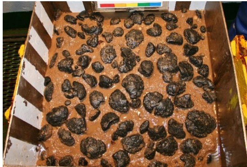
Figure 3. Polymetallic nodule sample collected during exploration, source: IOM, photo taken by T. Abramowski.
